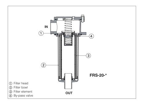
FRS return line filters are designed to protect pumps and the whole hydraulic circuit from contamination present in the working fluid.
